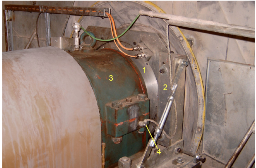
Large radial fan with installed balancing unit
