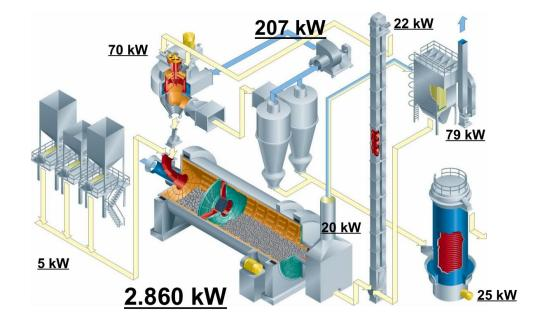
Example: a closed-circuit mill producing 104 t/h cement:
