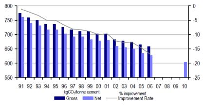
Reducing clinker factor and use of additives such as limestone, slag, fly-ash 0 & pozzolana can reduce energy consumption, CO<sub>2</sub> emission and production cost by as much as 50% or more.
