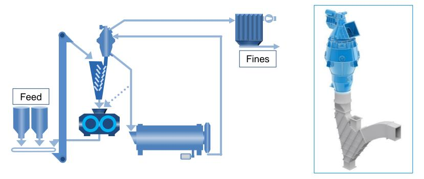
CPB single dynamic separator system reduces investment cost, plant complexity, and provides higher energy saving potential.
